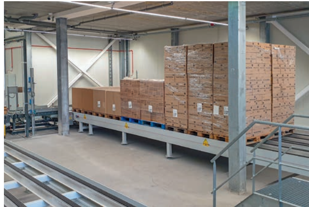
CargoMatic chain conveyor in Heavy Duty execution with 6 triplex chains.
